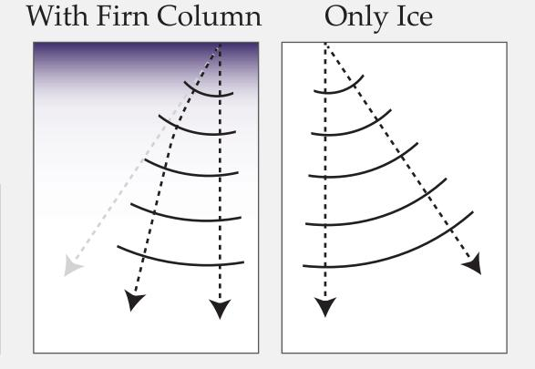
The corrections discussed here are all for a ground survey, using dipole antennae and a 3 MHz pulse frequency. Correction values will differ for surveys with a different radar configuration.
