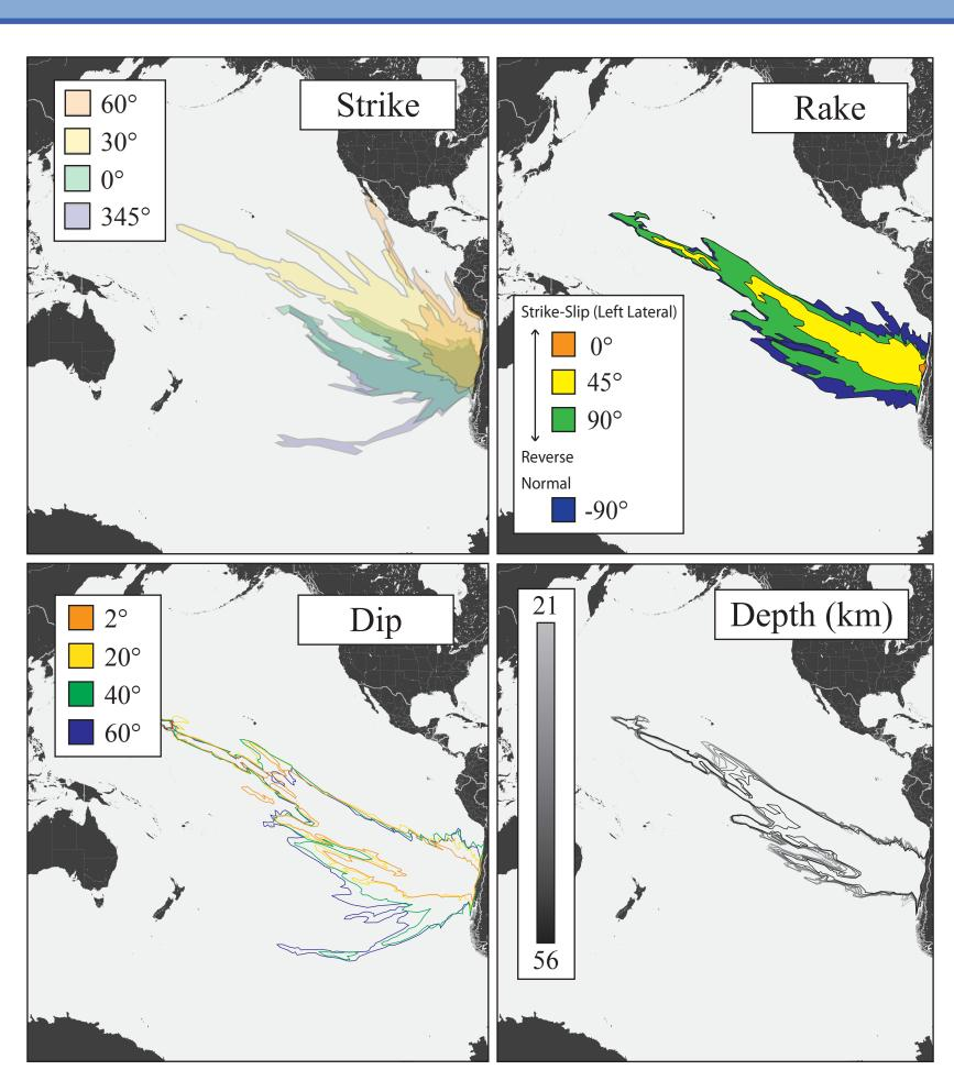
The above maps overlay the areas subjected to greater than 10 cm waves for a subset of the tsunamis modeled. The goal is to illustrate the effect of earthquake parameters on the size of the effected area and the directionality of the resulting tsunami. By plotting the data spatially, it makes it easy to determine if changes in tsunami severity exhibited by the time series data are global or local.
